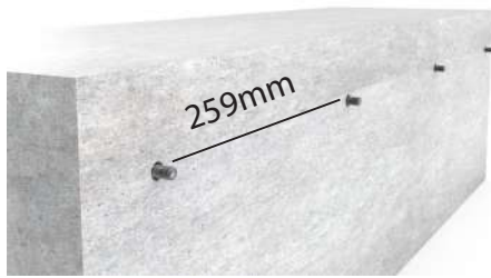
1. Drill, vacuum, insert glue and chemical anchor.
