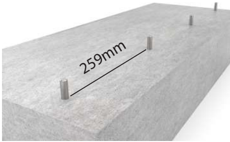
1. Drill, vacuum, insert glue and chemical anchor.
