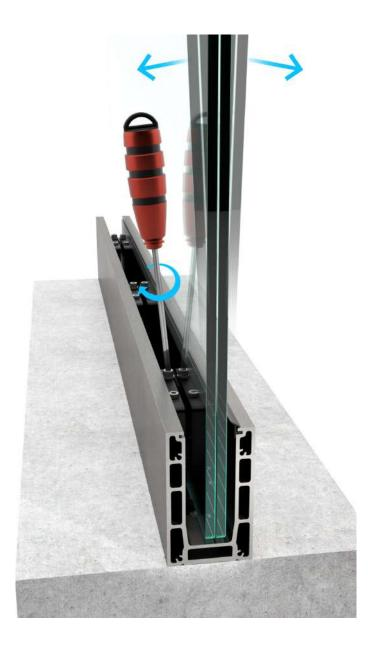
**TV8900** – is our innovative and most technically advanced glass railing. With over 15 months of development and prototyping, we were able to deliver ease of installation to a whole new level. Precise alignment of the glass is made from the safety of the inside of the balcony with just a hexagon M5 key, all done in seconds with an electric screwdriver. Its strength of up to 2kN using standard tempered laminated glass makes this system among the most desirable solutions on the Market.
