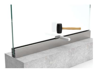
Once all wedges are in place, use wedge inserter and a hammer to insert them until the glass is locked.
