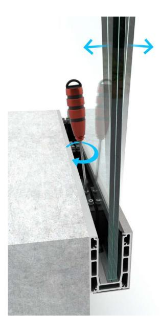
**TV8900S** – is our innovative and most technically advanced glass railing. With over 15 months of development and prototyping, we were able to deliver ease of installation to a whole new level. Precise alignment of the glass is made from the safety of the inside of the balcony with just a hexagon M5 key, all done in seconds with an electric screwdriver. Its strength of up to 2kN using standard tempered laminated glass makes this system among the most desirable solutions on the Market.
