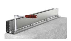
2. Place the profile and secure using a rachet spanner.
