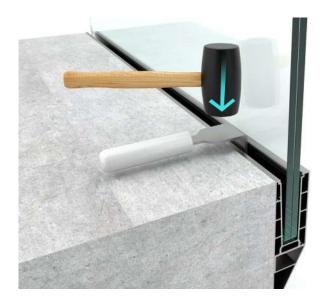
Once all wedges are in place, use wedge inserter and a hammer to insert them until the glass is locked.
