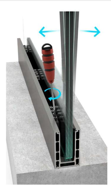
**TV9900** – is our innovative and most technically advanced glass railing. With over 15 months of development and prototyping, we were able to deliver ease of installation to a whole new level. Precise alignment of the glass is made from the safety of the inside of the balcony with just a hexagon M5 key, all done in seconds with an electric screwdriver. Its strength of up to 4kN using standard tempered laminated glass makes this system among the most desirable solutions on the Market.
