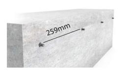
1. Drill, vacuum, insert glue and chemical anchor.
