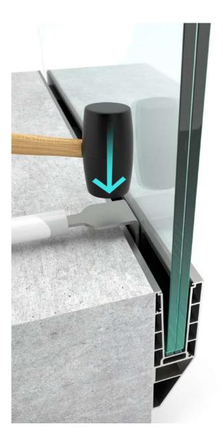
**TV7600Y** is our newest in-house designed Y-shaped glass railing system for side mount. This budget-oriented system provides a sleek finish, ease of installation, and requires minimum maintenance. The glass is secured in seconds using wedges and a wedge inserter. The wedges and profile design are ridged to remove the possibility of loose wedges which is a common problem with this type of design. You can rest assured that even after heavy use the system will keep its integrity.
