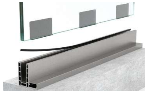
4. Place back rubber seal, back plastic inserts and laminated glass.
