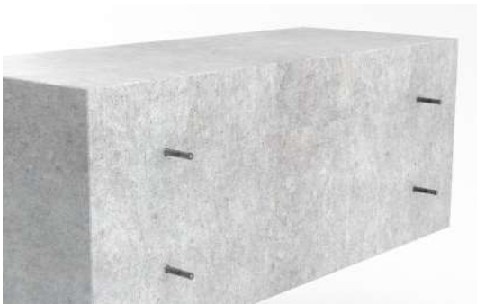
1. Drill, vacuum, insert glue and chemical anchor.
