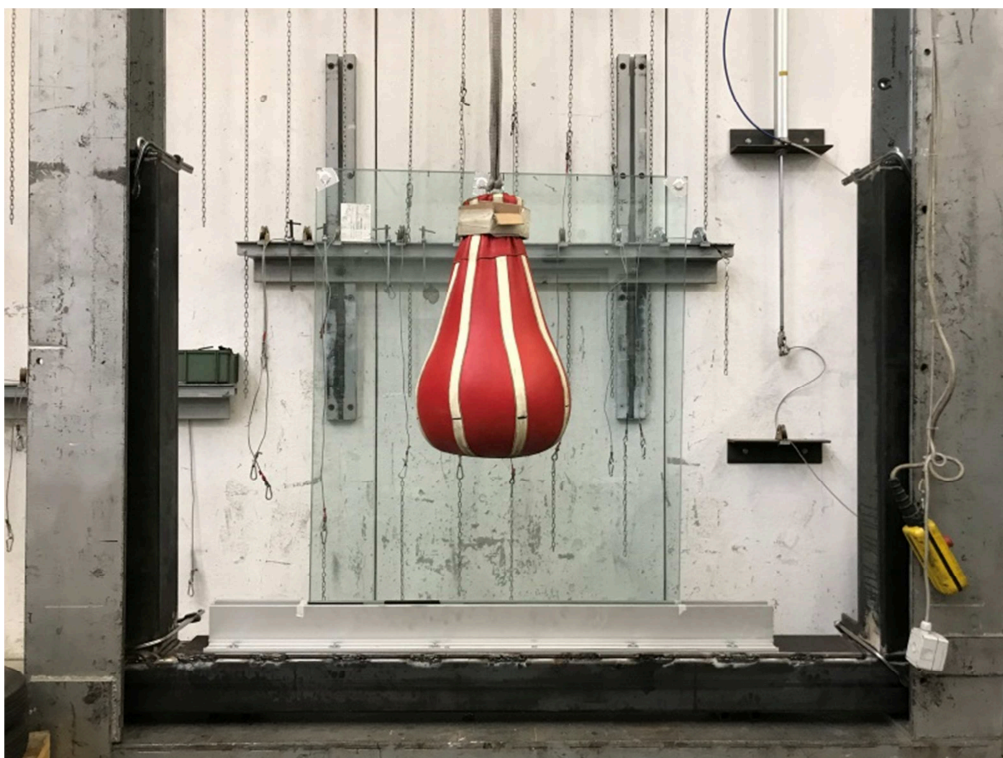
Photograph of the item after impact on the centre of the glazing with dynamic load according to standards UNI 10807:1999 and NF P01-013:1988
