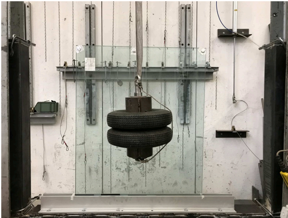
Photograph of the item after impact on the centre of the glazing with dynamic load according to standard UNI EN 14019:2016
